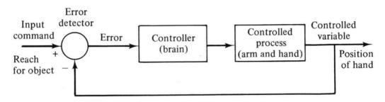
Figure 4: Block diagram of a human being as closed-loop control system [1]
